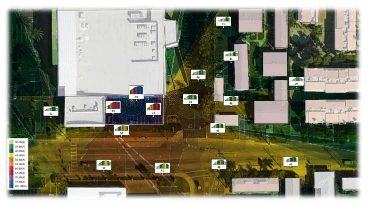
The final simulation is using a 12-foot-high wall/acoustic barrier:
