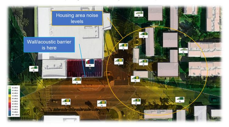
Note that housing area levels have dropped to around 50 dBA- the noise limit for after 11 PM usage.
