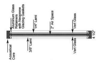
The glass area will have slightly less noise blocking ability compared to concrete block constructionhowever, the wall structures and the fact that only low-level ambient music is planned in the outdoor area, will allow for good noise compliance.
