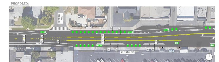
CONCEPTUAL FOR PLANNING PURPOSES NOT FOR CONSTRUCTION W 19TH STREET AT FEDERAL AVENUE CONCEPTUAL STRIPING PLAN
