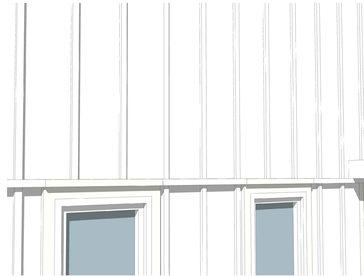
2 VERTICAL BOARD & BATTEN SIDING
