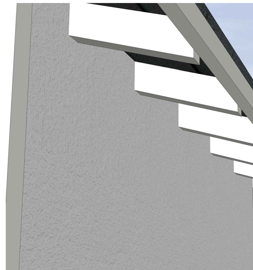
7 EXPOSED TRUSS TAILS W/ 2X3 FASCIA BOARD
