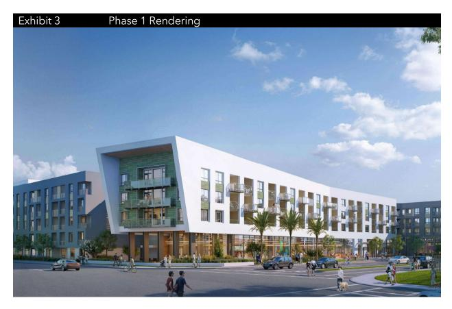
As shown in exhibit 3 above, Phase 1 incorporates modern architectural elements including large open storefront windows at the public spaces, and modern building materials including stucco, wood like fiber cement siding, metal paneling, stone tile, glass guardrails, and metal accents. The southeast corner of the project includes a publicly accessible plaza area with direct access to the retail component. Artwork is proposed throughout the plaza and within the building itself.
