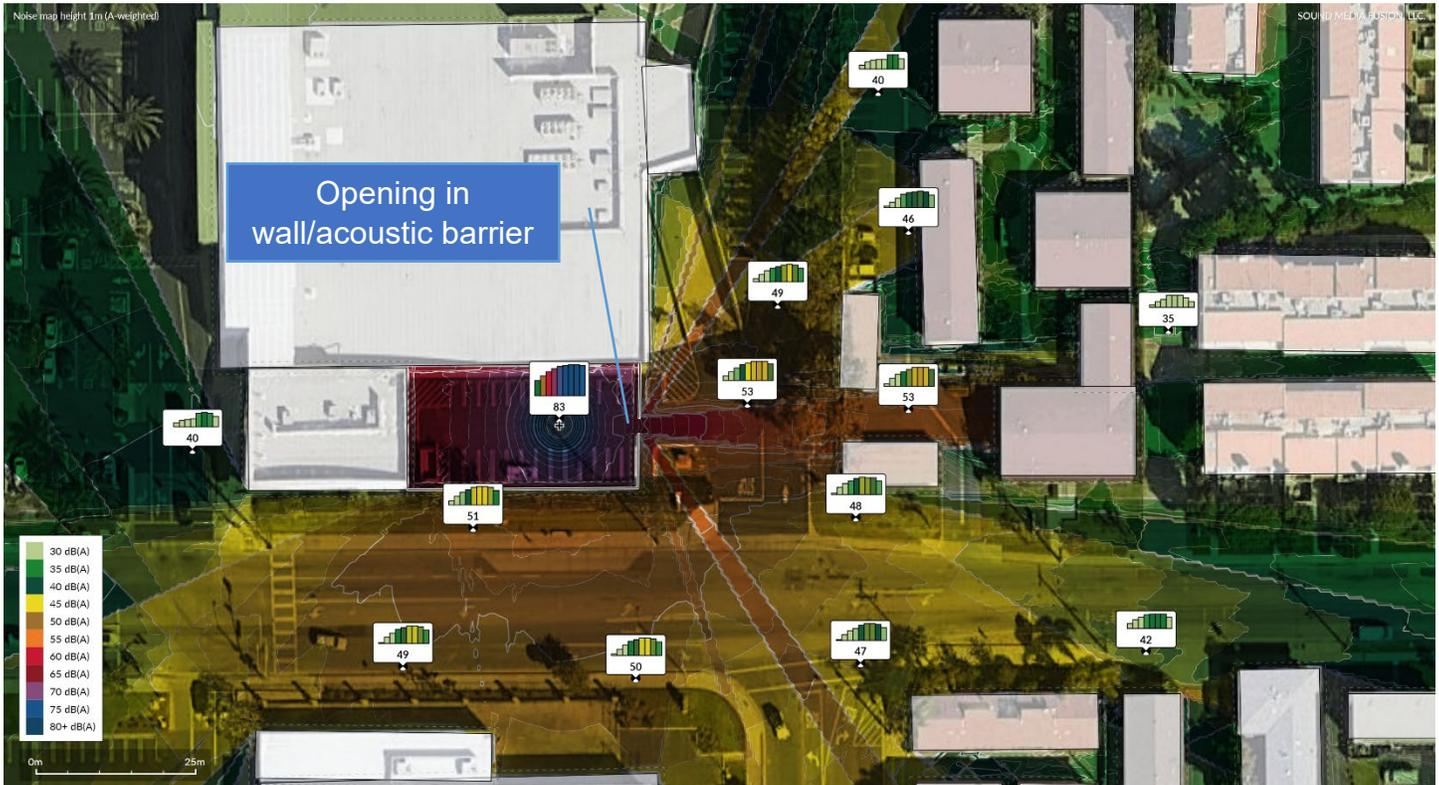
The opening in the wall/acoustic barrier is allowing sound to propagate into housing areas- note the level increase (53 dBA) in the acoustic path of the open door, with the color field showing the acoustic path of the noise.
