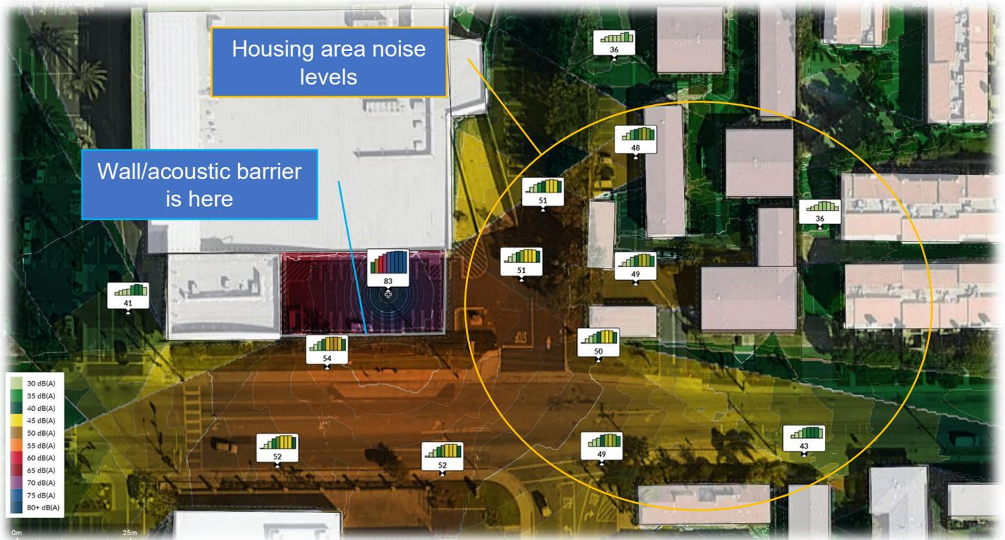
Note that housing area levels have dropped to around 50 dBA- the noise limit for after 11 PM usage. Housing area levels are more acceptable, even though the sound system is not yet in an optimum location. You can clearly see, based on the color sound field display, how sound is more contained within the confines of the venue, via the acoustic barrier. Venue sound system is operated at a lower (much less ideal) sound level in this simulation- in order to try and meet noise compliance.
