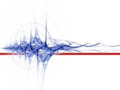
The next simulation is as above, with a 'door' (open) in the barrier, showing resulting noise higher in an area near the door, and past to door- indicating the importance of a relatively 'sealed' barrier:
