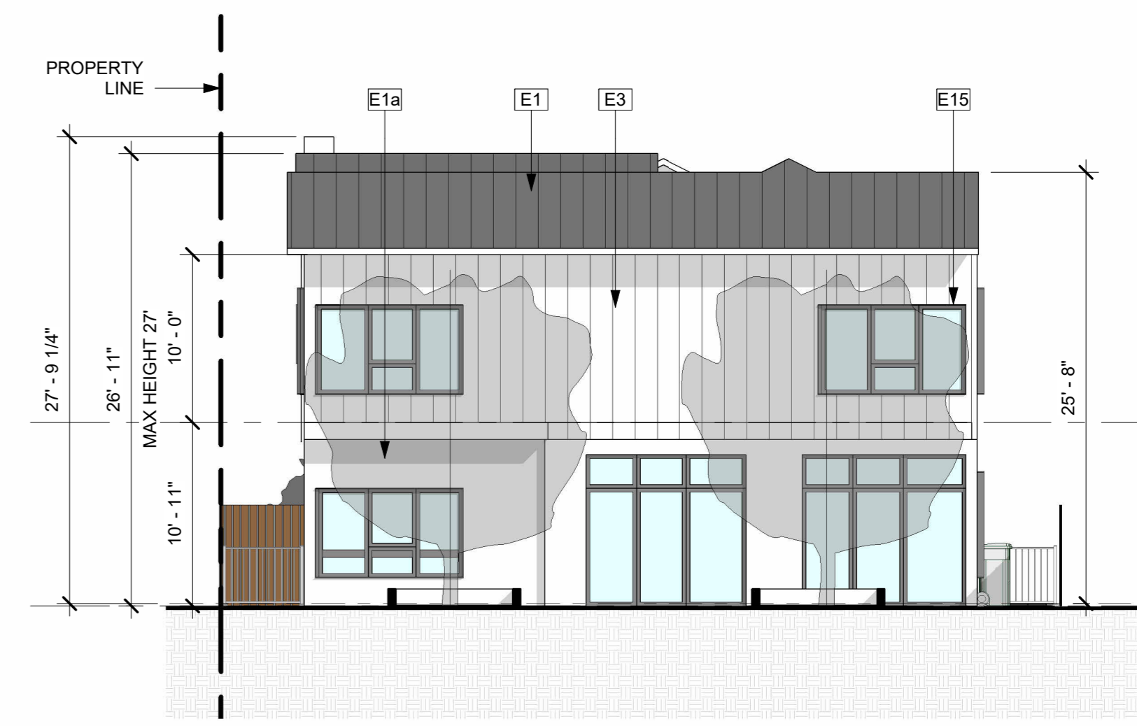
NORTH ELEVATION (REAR)
