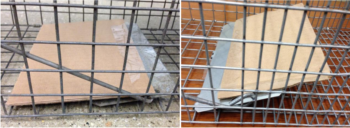
A cardboard extender for a short trip plate decreases the chance of a cat stepping or reaching over the trip plate to eat the bait without getting trapped. You can tape the extender either to the front of the plate (left) or to the rear (right). Photo credit: ASPCA
