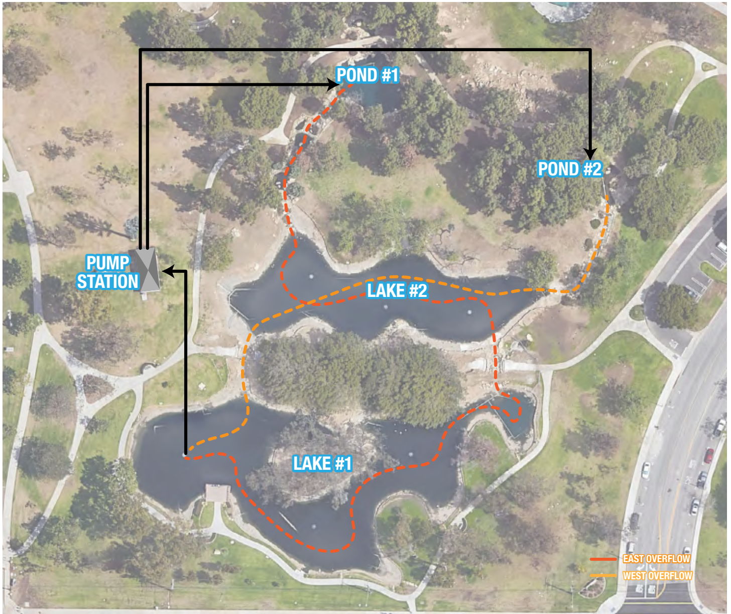
Conceptual circulation flow routing layout that minimizes piping and optimizes circulation for water quality benefit.
