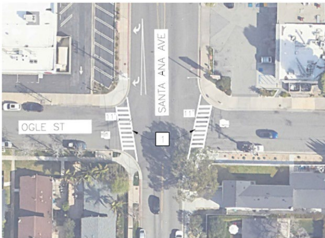
NEW CROSSWALK MARKINGS AT SANTA ANA AVE. & OGLE ST.
