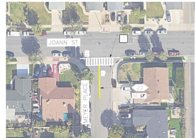
NEW CROSSWALK MARKINGS AT JOANN ST. & MEYER PLACE
