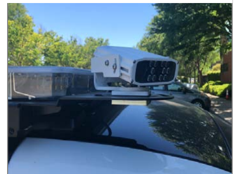
Figure 11. Mobile LPR Camera
