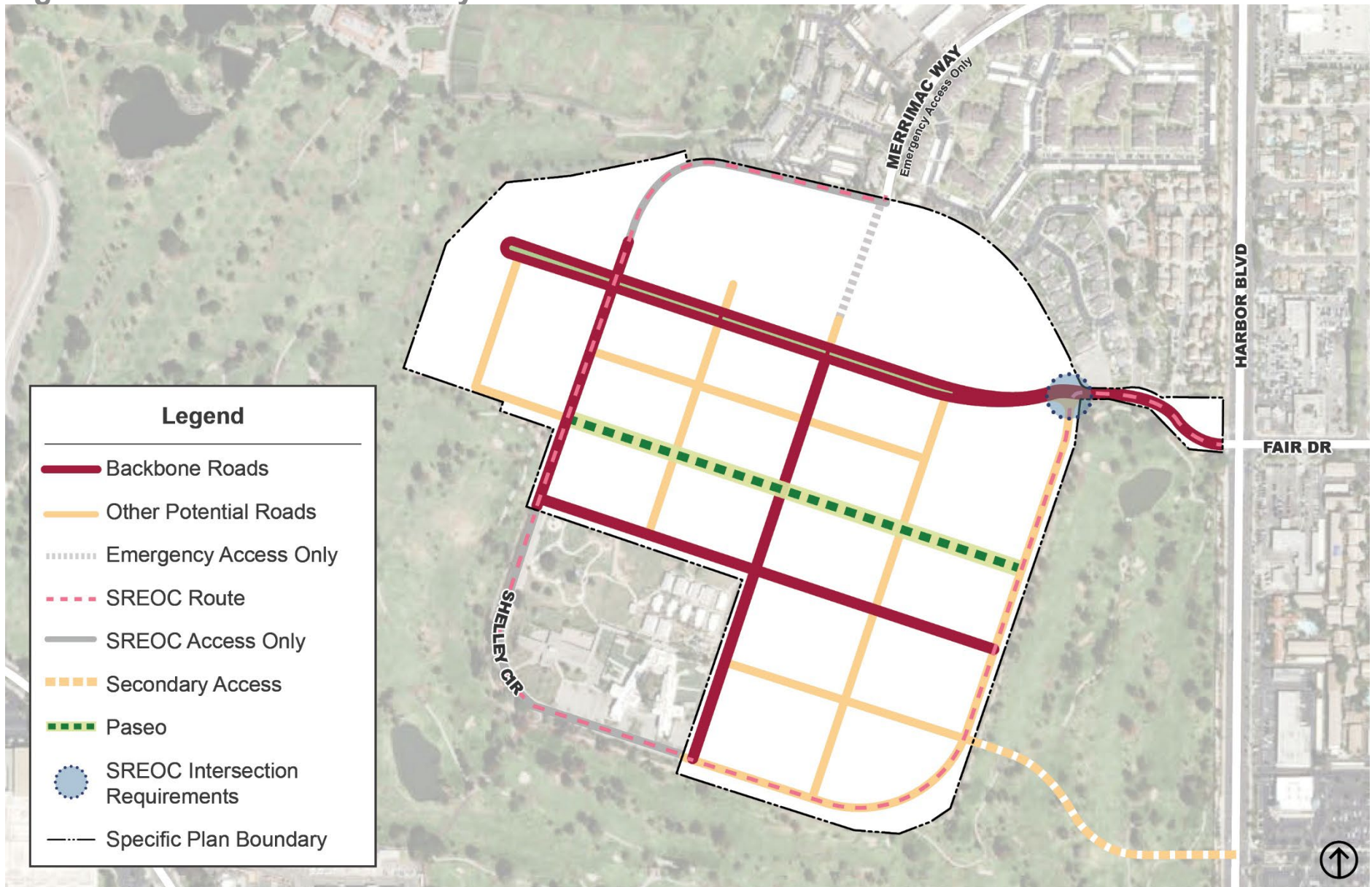
Figure 5-3: Backbone Roadway Network
