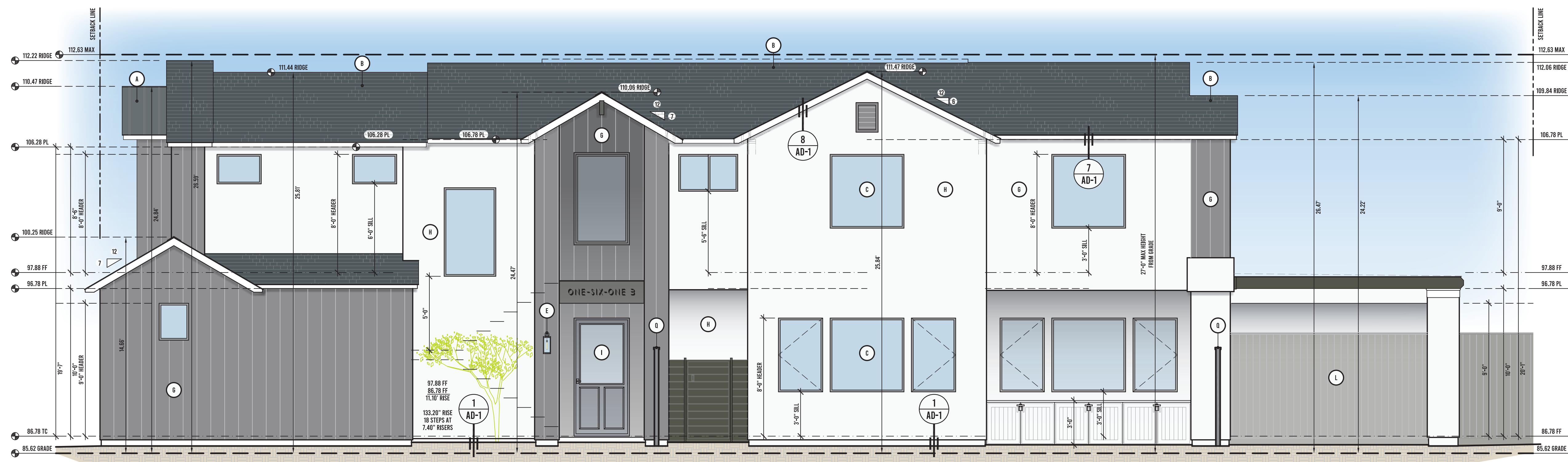
RIGHT ELEVATION - UNIT B
