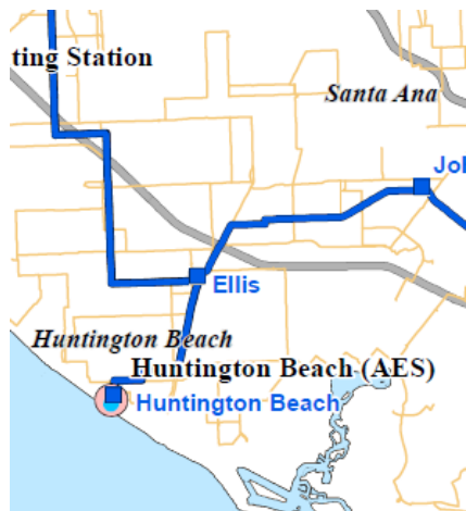
Figure 3-4: Transmission lines of power for Costa Mesa, originating in the Huntington Beach (AES). Blue Line: 220-287KV, Gold Lines: 110-161KV. Source
